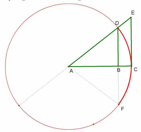
In this diagram  $\angle A$  will refer to the angle  $\angle EAC$ Circle A is a unit circle. (i.e. AC = 1)  $\triangle ABD \sim \triangle ACE$  so we know that all corresponding ratios are EQUAL.
